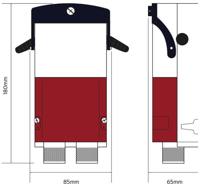
DP single phase, single fuse with earth block and brass plate. 2 x 25mm tubes
